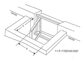
Window wells with a vertical depth greater than 44 inches below the adjacent ground level shall be equipped with a permanently affixed ladder or steps usable with the window in the fully open position. The
